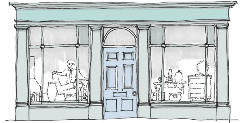
2. The Georgian shopfront often infilled the colonnade with glazing and stallriser between the bases, keeping the classical appearance
