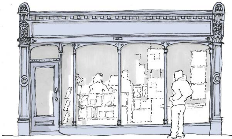
3. A Victorian approach introduced many variations and embellishments of detail, such as ornate console brackets, dentilled cornices, decorative transoms and mullions and panelled fascia and pilasters
